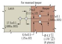
For right angle keeper Ø 4.3 <sup>+0.1</sup><sub>-0.0</sub> (.170 <sup>+.003</sup><sub>-.001</sub>)  $17.5 \pm 0.1$ (.688±.005) Four holes Latch sub-ass'y 72±3 mounting holes  $(2.82 \pm .12)$  $12^{+6}_{-0}$  $(.46^{+.25}_{-.00})$ Keeper mounting holes >  $6.4 \pm 0.5$  $12.7 \pm 0.1$  $(.25 \pm .02)$  $(.500 \pm .005)$
