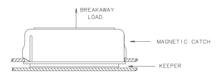
THE FOLLOWING TEST DATA APPLIES TO THE 02-10-20X-X0 MAGNETIC CATCHES AND THE 02-14-102-11 KEEPER.
