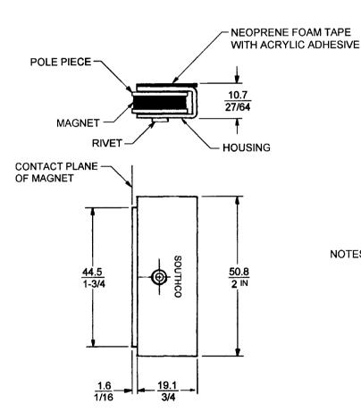
TO INSTALL REMOVE PROTECTIVE PAPER AND APPLY ASSEMBLY TO A CLEAN, DRY SURFACE
