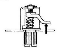
FASTENERS YIELDED WHEN A LOAD OF 100 LBS. WAS APPLIED IN THE DIRECTION OF THE ARROW. HOWEVER FASTENER COULD NOT BE UNLATCHED WITH THE LOADS INDICATED IN THE FOLLOWING TABLE.
