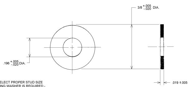
NOTE: TO SELECT PROPER STUD SIZE WHEN SEALING WASHER IS REQUIRED - ADD THICKNESS OF WASHER (.019) TO TOTAL THICKNESS OF MATERIAL TO BE FASTENED.
