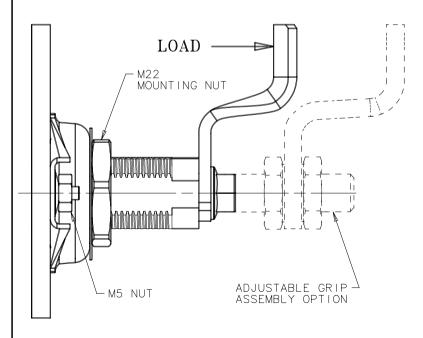
COMPRESSIVE STRENGTH - MAXIMUM WORKING LOAD: 445 N (100 lbf) \* - AVERAGE ULTIMATE LOAD: 1112 N (250 lbf) \*
